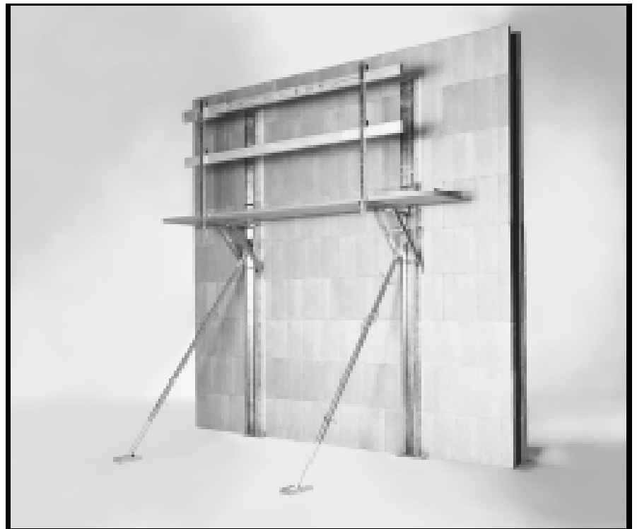
Third Course and Wall Alignment Installation
