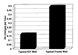
The interlocking foam faces, sealed with continuous concrete in the center, make ICF walls exceptionally airtight. So drafts are cut sharply. In tests, houses built of ICFs had up to one-third to one-half as much air infiltration as the typical frame house.
