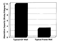
The heavy concrete of the ICF wall gives it the heat-absorbing property of "thermal mass". This smooths out swings in temperature over time. So the house does not tend to overheat or get suddenly chilly as the furnace or air conditioner cycles on and off.
