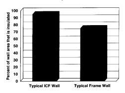
The continuous layer of foam insulation along the ICF wall helps keep the temperature the same everywhere. It virtually eliminates the "cold spots" that can occur in frame walls along the studs or at gaps in the insulation.
