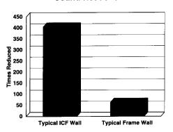
Compared to a typical wood frame wall, only about one-quarter to one-eighth as much sound penetrates through an ICF wall. Scientists would describe loud speech on the opposite side of a frame wall as "audible, but not intelligible." On the opposite side of an ICF wall, a listener would "strain to hear" loud speech. It would be virtually "inaudible."
