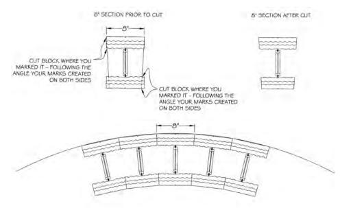
**Step 7**: Zip tie the blocks together. Additional reinforcing in the form of flexible, hardboard / masonite should be attached to the outside of the wall.
